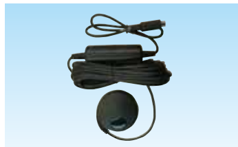
●GP5001 GPS receiver Improves the frequency stability from 0.1ppm to +/- 0.01ppm, by using the GPS pulse signal for an accurate time base of the local oscillator circuit.
