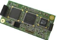
**Ethernet controller - ARL2300**: Allows remote control, 10MHz spectrum display, remote listening and audio recording of your AR6000 receiver, through the local network and Internet. Selectable audio bit rate.
