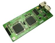
**GPS receiver – GP5001**: Improves the frequency stability of AR6000 from +/- 0.1ppm to +/- 0.01ppm, by using the GPS pulse signal for an accurate time base of the local oscillator circuit.
