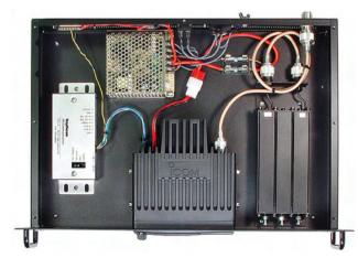
Clean and simple layout is easy to access and maintain. Receiver, pilot tone generator, and power supply, all in one chasis.
