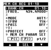
3. Use the [▶] button to move to the last line [MEM CH PARAM SET] and press [ENT].
