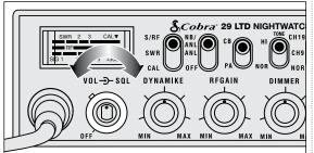
3 To achieve the Desired Squelch Setting (DSS), turn the Squelch control (a) counterclockwise until you hear noise. Now turn the control clockwise just until the noise stops. This is the DSS setting.
