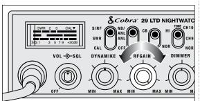
• Rotate the © RF Gain knob counterclockwise to reduce gain in strong signal areas. In weak signal areas turn clockwise to increase gain.
