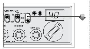
**1** Switch to NOR to select desired channel.
