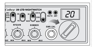
While holding mic button adjust the SWR CAL knob so the meter needle swings to the CAL ▼ mark on the meter (located on the right).
