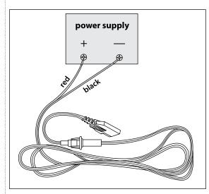
Simply connect the red (+) and black (-) leads of the transceiver to the corresponding terminals of the power supply.
