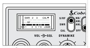
1 The S/RF-SWR-CAL switch must be in the S/RF position to read the meter.
